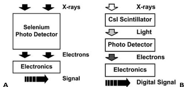
**Figure 2.9** Indirect and direct digital (flat-panel) image receptors. The indirect (left) detector uses a CsI scintillator, virtually identical to that in an image intensifier, to convert the x-ray signal into light. A photodetector converts the light into an electron signal. This signal is then digitized. The direct detector (right) uses a selenium layer to directly convert the x-ray signal into an electrical charge distribution. This signal is then digitized.
