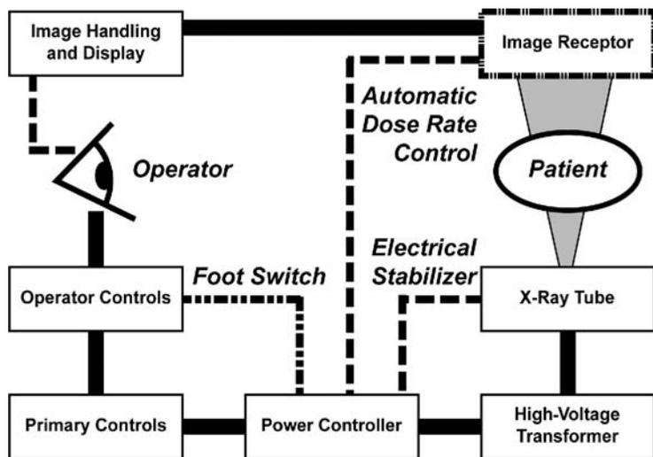
**Figure 2.4** Generator and feedback schematic. Modern generators rely on a large number of feedback loops to manage radiation dose and stabilize image quality. The operator provides the final control loop by managing system resources.
